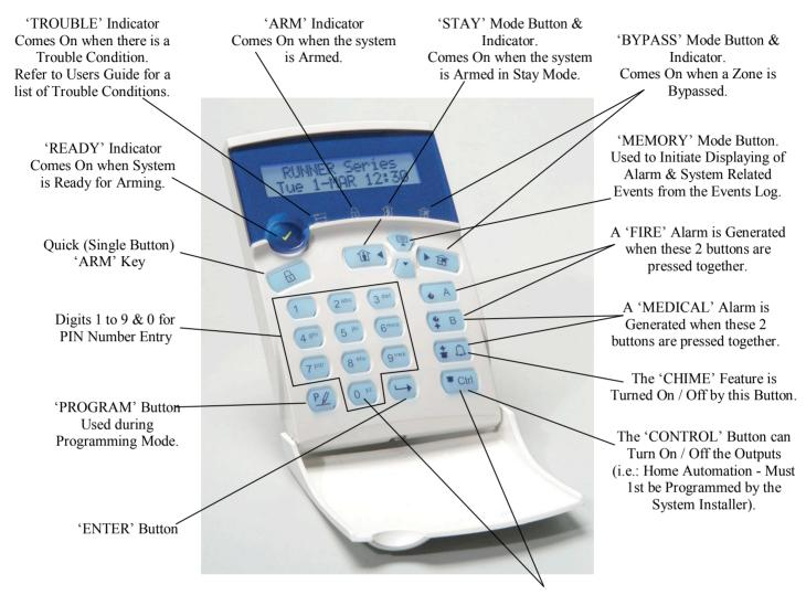
The 'CONTROL' & '0' Buttons Pressed Together During Programming will Clear (Delete) the content of a programming location such as Phone Numbers, Wireless Codes, etc. The Enter Button Must then be pressed to confirm the deletion.
